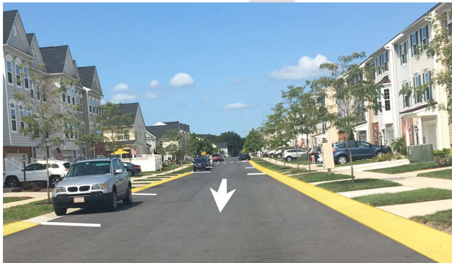
Figure 3B. Example of a street with one-way traffic and parking on both sides
